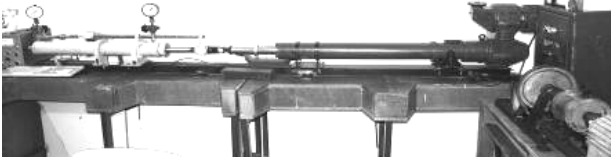
Fig. 6. The trial stand of industrial linear actuator.
