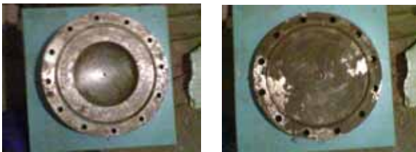
Fig.4. First stage experimental sheet deforming mould through hydroformation.
