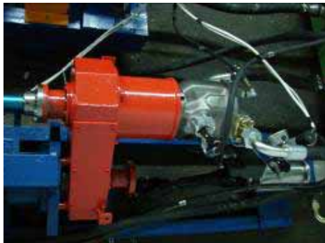
Fig. 9. The hydro-mechanical module.
