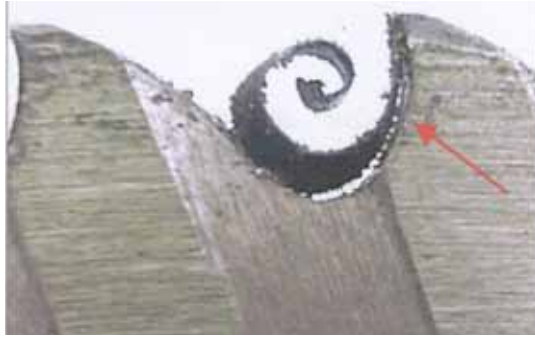
Fig. 2. The creation of scobs during the cutting process with saw [1].
