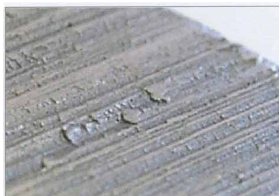
Fig. 7. Detail of cut surface after cutting with circular saw: steel ISO Fe510 [1].
