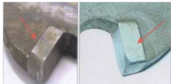
Fig. 4. The detail of the embedded cutting teeth [1].
