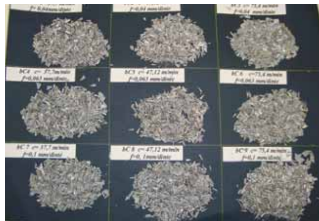
Fig. 3. Chip forms in drilling.
