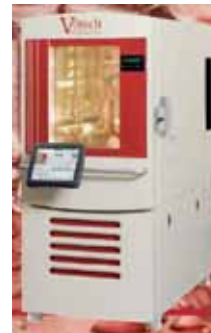
Fig. 6. Climatic furnace Vötsch.
