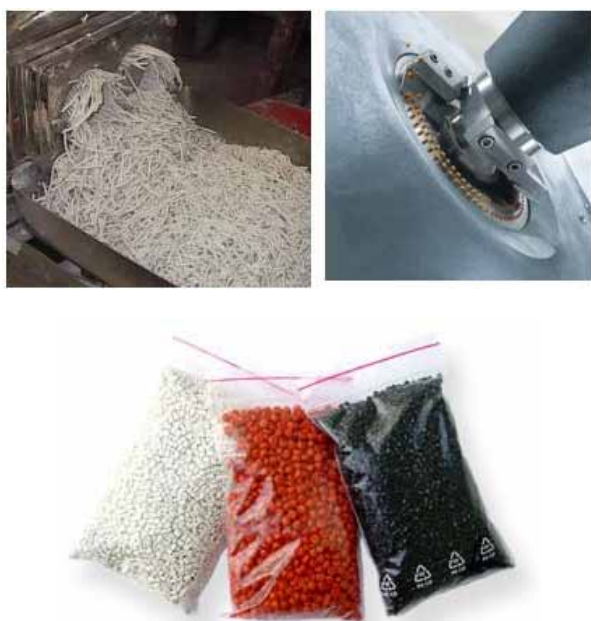
Fig. 3. Regranulate and original stock (polycarbonate).
