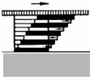
Fig. 2. Flow between two parallel plates [5].
