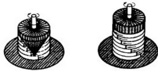
Fig. 5. Flow between a cone and plate or Flow between two parallel plates [5].
