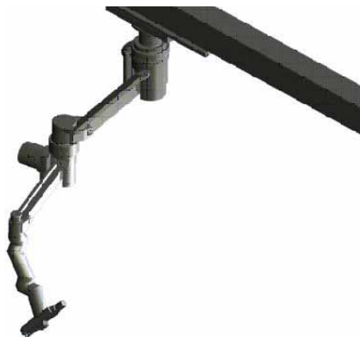
Fig. 15. The suspended surgical robot.
