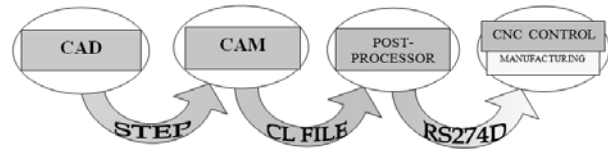
Fig. 2. Data flow from CAD to manufacturing.
