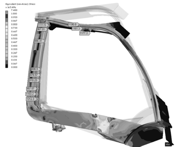
Fig. 9. Equivalent stress distribution for load case 3.
