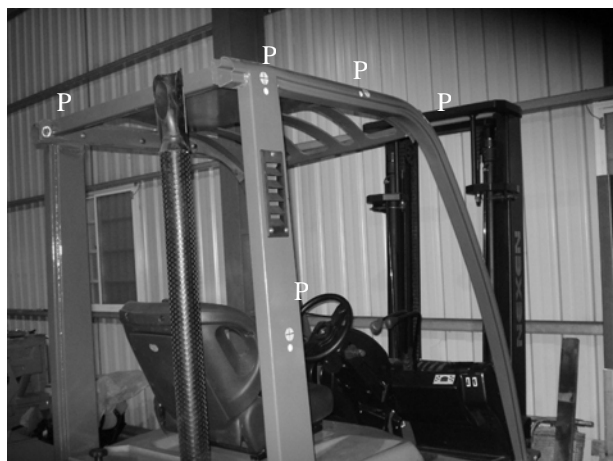
Fig. 11. Characteristic points for measurement.
