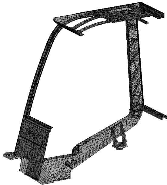
Fig. 5. Examined FE model of final OHG design.
