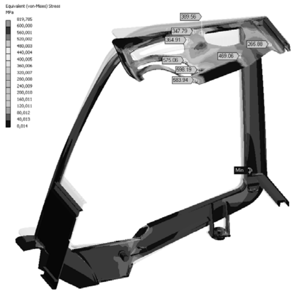
Fig. 8. Equivalent stress distribution for load case 2.
