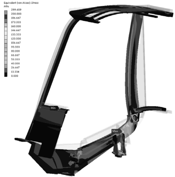
Fig. 7. Equivalent stress distribution for load case 1.
