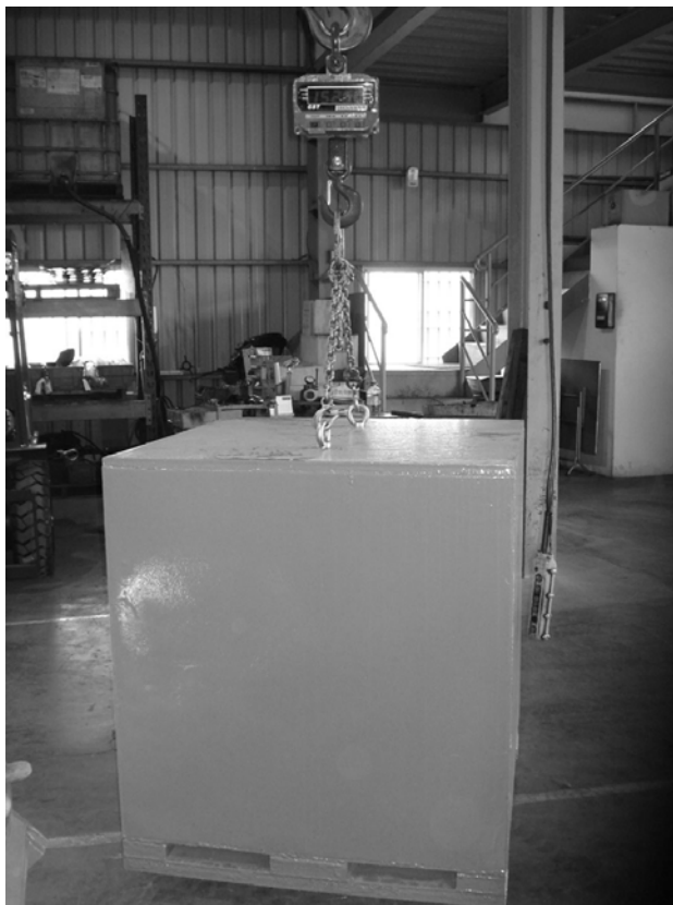
Fig. 10. Impact drop test sample load.
