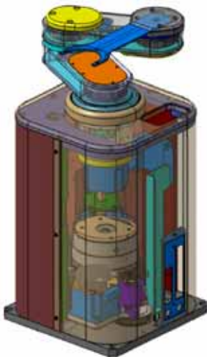
Fig. 9 – SCARA-type robot designed for wafer manipulation in atmospheric environment.
