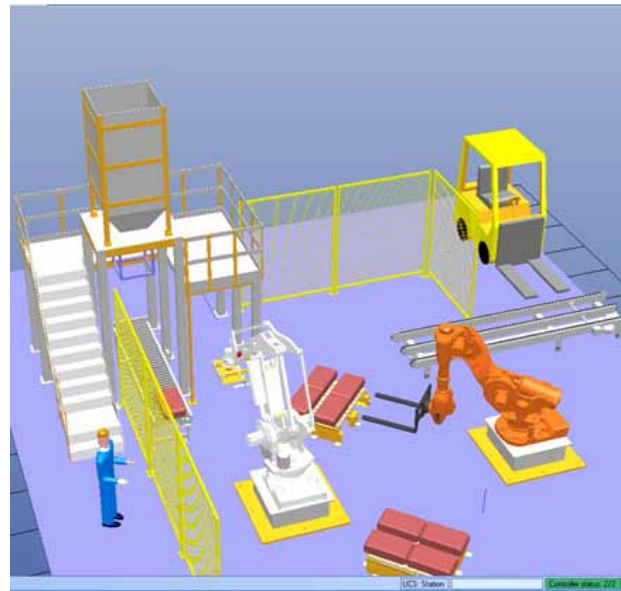
Fig. 1. Complex palletizing system.
