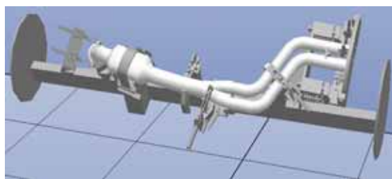
Fig. 4. Exhaust gas piece and fixture devices.
