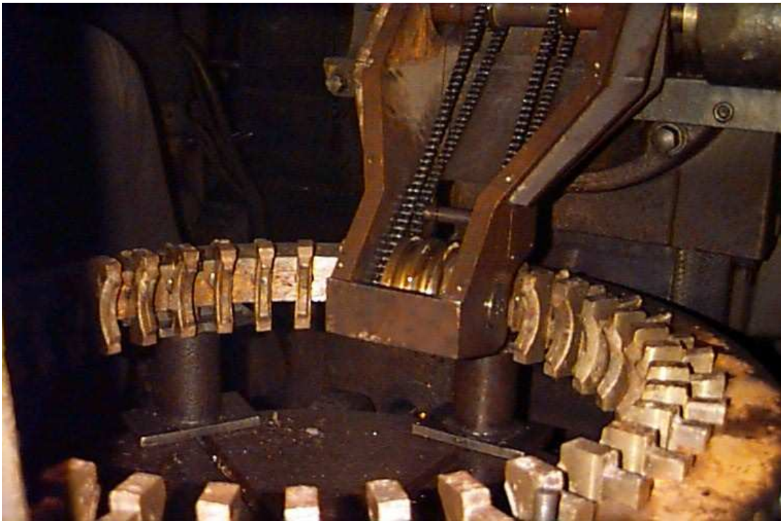
Fig. 14. The helical worm–internal teeth worm wheel drive.
