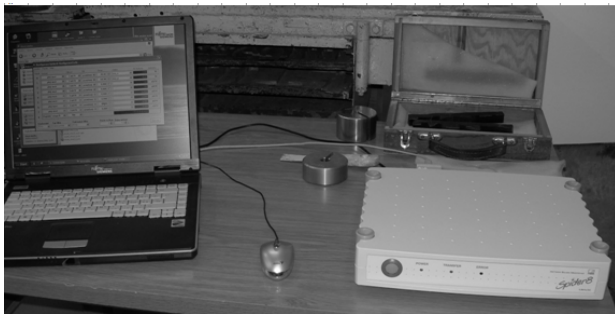
Fig. 5. Measuring device for cutting forces in machining type Conmes Spider along with evaluation software and PC components of cutting forces depending on cutting parameters.
