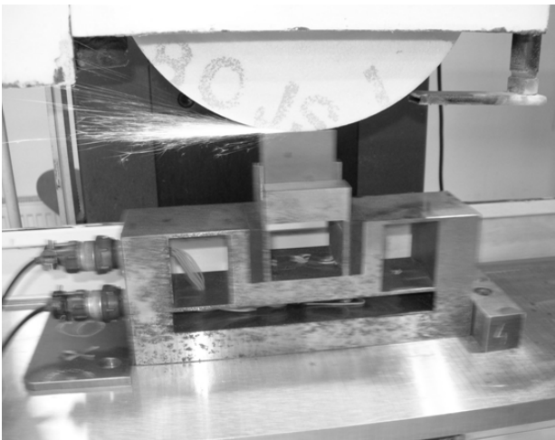
Fig. 2. Surface grinding of the sample circuit blade clamped in a two-component strain-gauge dynamometer.
