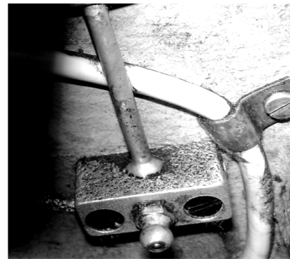
Fig. 13. Grease nipple with ball.
