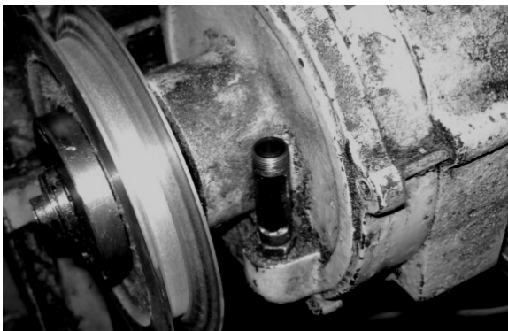
Fig. 2. Motor reducer with oil bathroom system.
