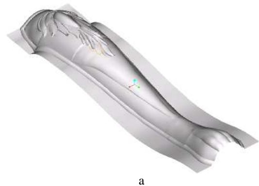
Fig. 5. Free form surface creation through the boundaries and curves (yellow color) using advanced blend option.
