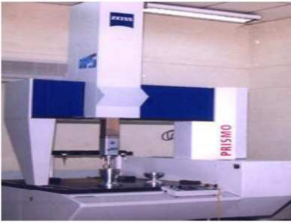
Fig. 2. ZEISS-Prismo5 3D Co ordinate Measuring Machine.
