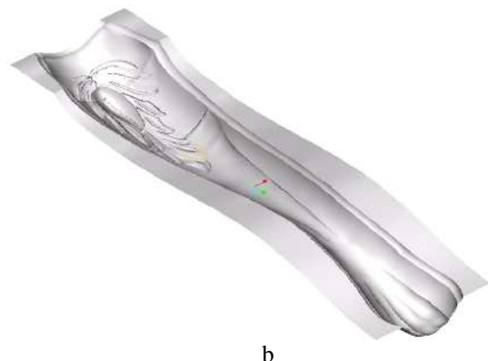
Fig. 6. (a)(b) Final surface model development using advanced surfacing features in Pro/Engineer.
