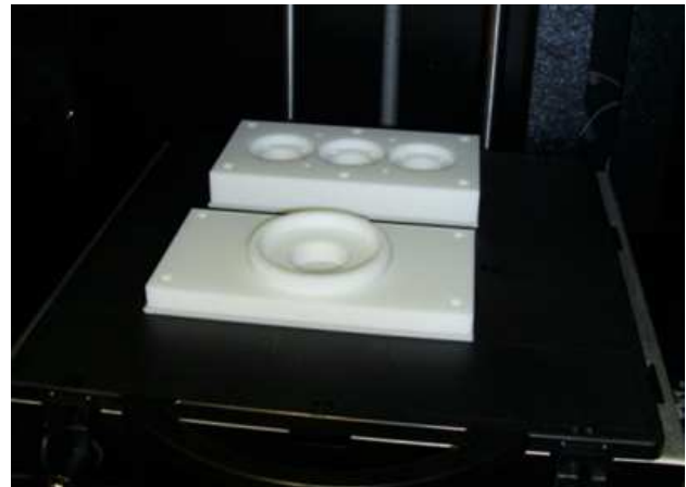
Fig. 5. Printed prototype of 3D part by FDM method.
