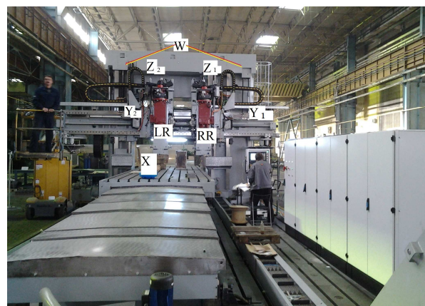
Fig. 8. View of the milling machine with displaceable table FLP 2200 CNC type: a – ram details; b – general view; X , Y_1 , Y_2 , Z_1 , Z_2 – numerically controlled axes, W – positioning axis, 1 – bed, 2 – displaceable table (it travels on X axis), 3 – feed kinematic chain of the table, 4 – columns, 5 – crossrail balancing cylinders, 6 – cross-rail, 7 – cross beam, 8 – pulleys system, 9 – kinematic chain for crossrail positioning (positioning on W axis), 10 – feed kinematic chains for left and right rams ( Z_1 and Z_2 axes), 11 – balancing cylinders of the two rams, LR – left ram, RR – right ram.
