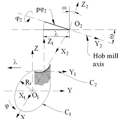
Fig. 2. The reference system of the hob mill,  $X_2Y_2Z_2$ .
