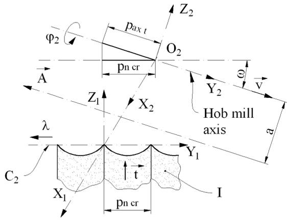
Fig. 3. The rack-gear normal pitch and the hob mill axial step.
