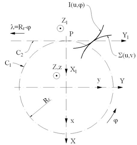
Fig. 1. The centrodes of  $\Sigma(u, v)$  and  $I(u, \varphi)$  surfaces.
