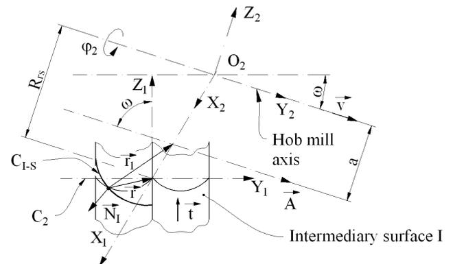
Fig. 4. The  $\vec{A}$  axis projection onto  $I$  surface.
