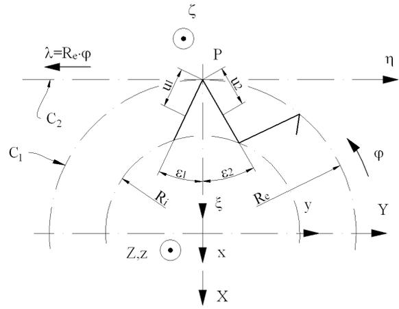
Fig. 5. The slitter saw cutter tooth profile.
