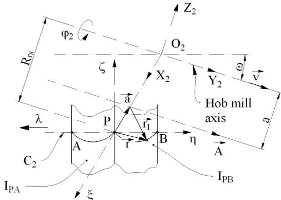
Fig. 6. The hob mill profiling.
