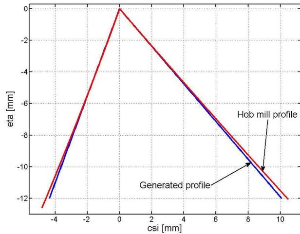
Fig. 7. The hob mill profile in axial section –  $S_A$ .
