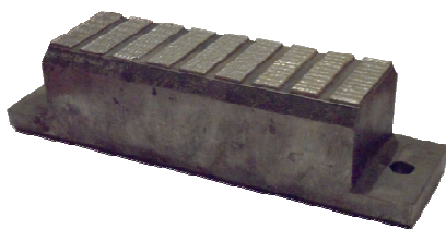
Fig. 3. Real workpiece with different cladded material zones.
