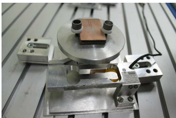
Fig. 2. The device for measurement of torque.
