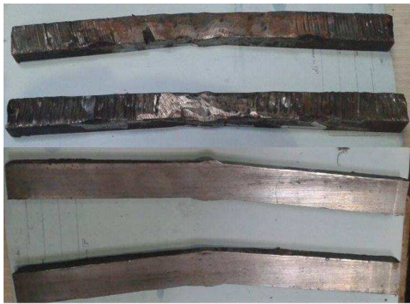
Fig. 1. Image with sampling from the beginning and from the end of the welded plate for homologating the welding process. (1:4 scale).
