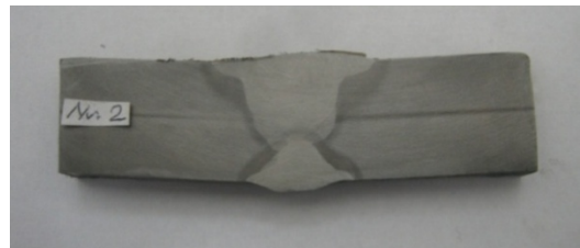
Fig. 2. Macroscopical image for the specimen cut off the beginning edge of the sample. (1:1.3 scale).
