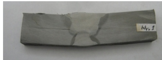
Fig. 3. Macroscopical image for the specimen cut off the end of the sample (the crater area). (1:1.3 scale).
