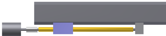
Fig. 6. CAD functional model of the radial feed drive of a turning machine for wheel sets.
