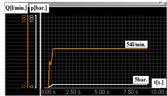
Fig. 4. Flow and pressure variation in the cooling unit on the outside of the tool
