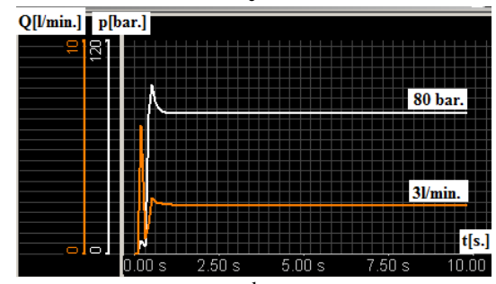
Fig. 5. Flow and pressure variation in the cooling unit on the inside of the tool: a – obstruction 0 %, the tool is withdrawn but the cooling unit is on, p = 5 bar and Q = 54 l/min; b – obstruction 50 %, the cutting process takes place with p = 18 bar and Q = 54 l/min; c – obstruction 75 %, the cutting process takes place with p = 66 bar and Q = 53 l/min; d – obstruction 99 %, the cutting process takes place with p = 80 bar and Q = 3 l/min.
