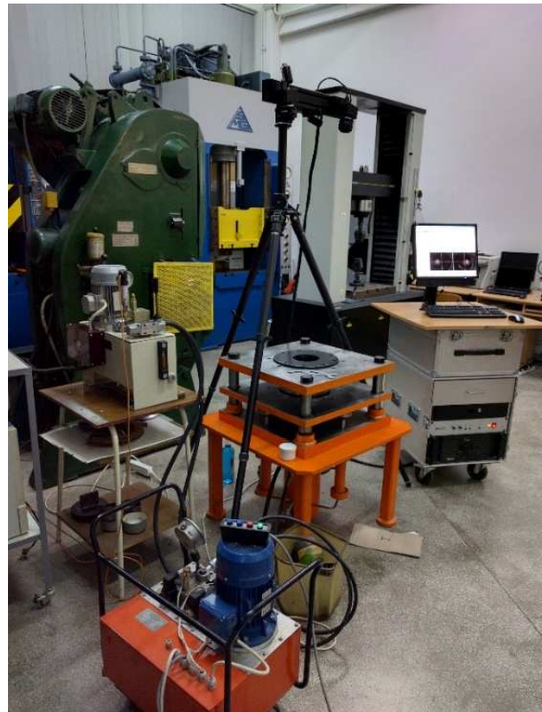
Fig. 6. Nakajima test experimental configuration – hydraulic high pressure unit (left), two CCD cameras mounted above the modular deep drawing unit (centre), GOM PC with Aramis software (right).
