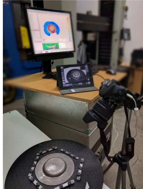
Fig. 15. Strain measurements on the drawn part with a DSLR camera connected to a tablet and analysed by Argus.
