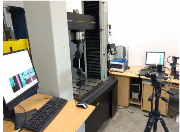
Fig. 3. Tensile test experimental configuration – GOM PC with Aramis software (left), Instron 5587 (centre), two CCD cameras (right front), PC with Blue-hill Software (right back).
