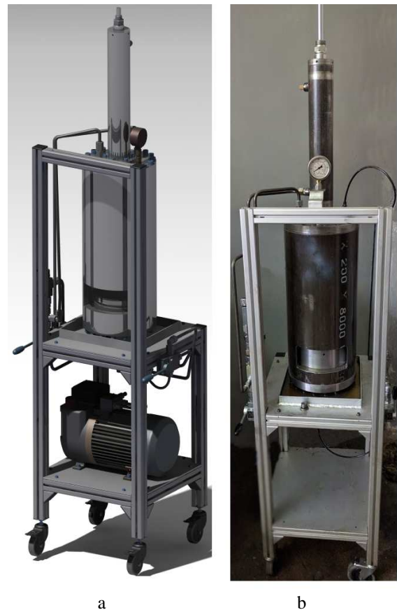
Fig. 11. Unique hydroforming solutions, concept developed by the authors: a – CAD developed concept; b – Physical developed concept.
