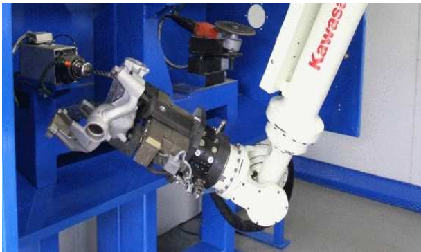
Fig. 2. Deburring application with the robot manipulating the workpiece.
