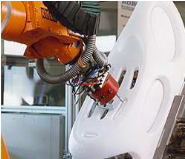
Fig. 1. Deburring application with the robot manipulating the tool.
