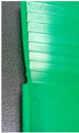
Fig. 19. Breaking of the part edge at the end of the DE segment on the conventional milling trajectory.
