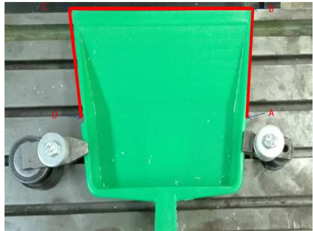
Fig. 13. Deburring the front part of the dustpan – conventional milling trajectory.
