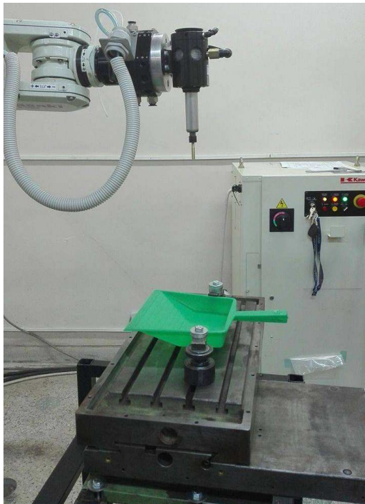
Fig. 12. Experimental setup for robotic deburring.
