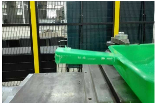
Fig. 16. Flattened burrs on the climb milling trajectory.
