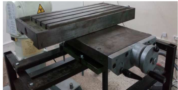
Fig. 10. The T-slot plate mounted on the two axis manual positioning system.
