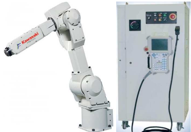
Fig. 4. Kawasaki FS10E articulated-arm robot and Kawasaki D controller.
