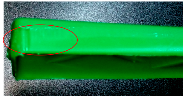
Fig. 17. Chipped part edge on the climb milling trajectory.
