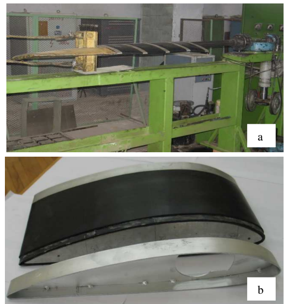
Fig. 3. Experimental set-up: a – stand for static tests; b – blade with flexible elements and rib.
