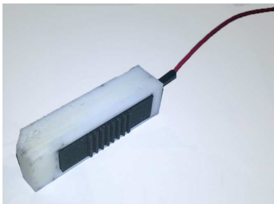
Fig. 4. 3D printed end-effector finger with capacitive touch sensing.
