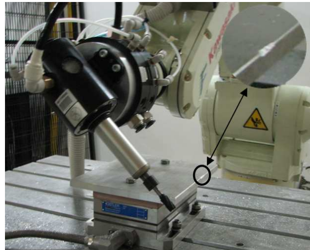
Fig. 9. The robotic chamfering operation; the gap used for evaluating the tool compliance behaviour can be seen on the edge of the part.
