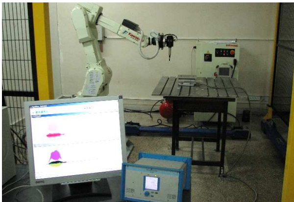
Fig. 8. The setup of the robotic cell.
