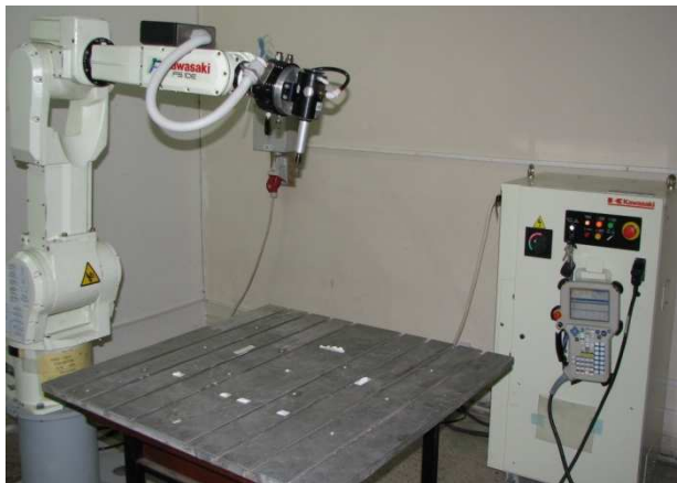
Fig. 5. Kawasaki FS10E articulated-arm robot and Kawasaki D controller.
