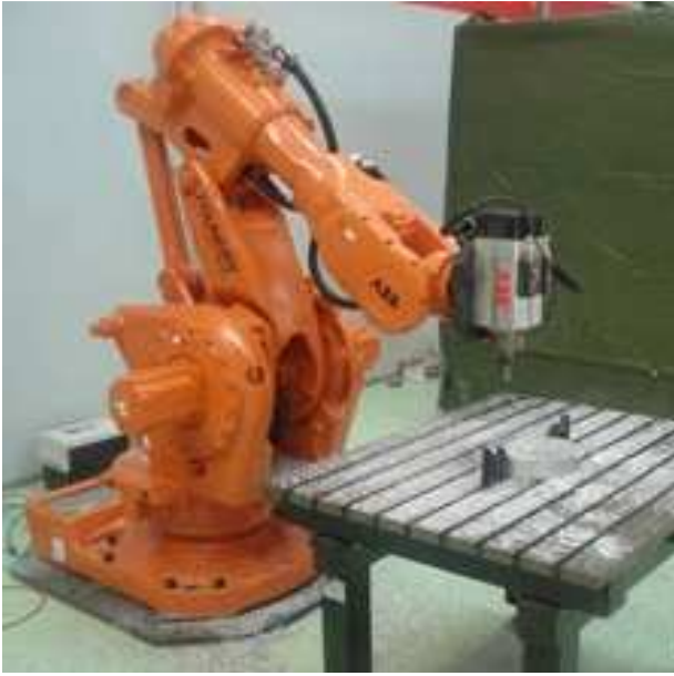
Fig. 1. Milling application with the robot manipulating the tool.
