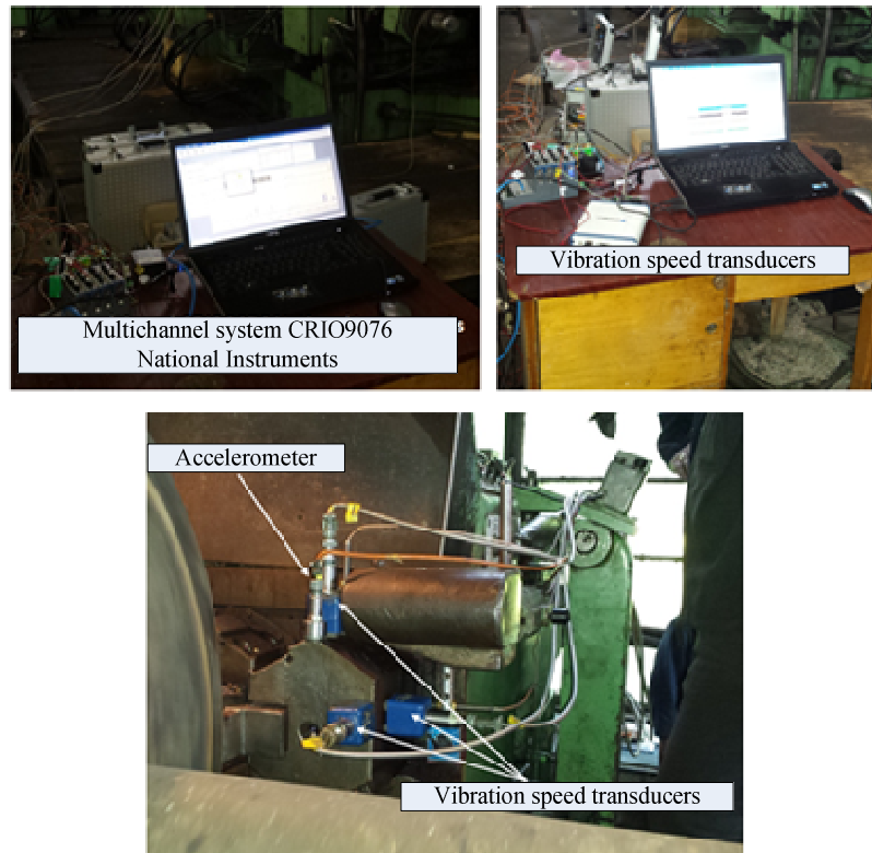
Fig. 2. Experimental set up.
