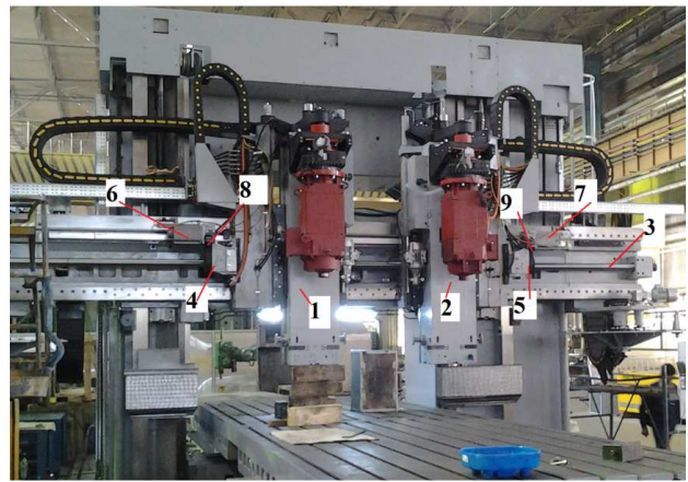
Fig. 14. Two speed drives with rotary nuts and fixed ball screw (1, 2 – slides moving horizontally; 3 – fixed ball screw; 4, 5 – rotary nuts; 6, 7 – feed electric motors; 8, 9 – toothed belts).
