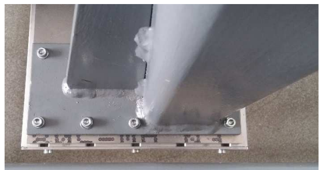
Fig. 5. System for adjusting the angle between X and Y axes.
