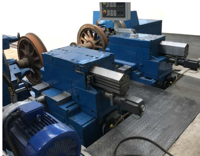
Fig. 7. Retrofitted lathe for re-profiling railway wheelset.
