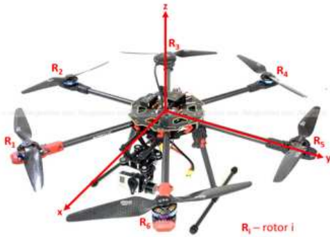
Fig. 5. The hexacopter coordinate system and numbering of the rotors.
