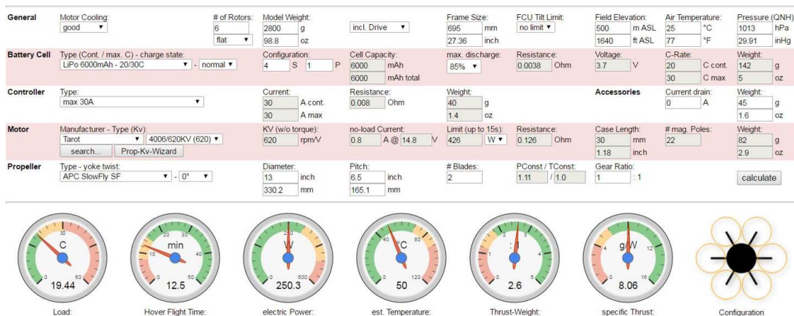
Fig. 13. Choosing the components that equip the drone [1].
