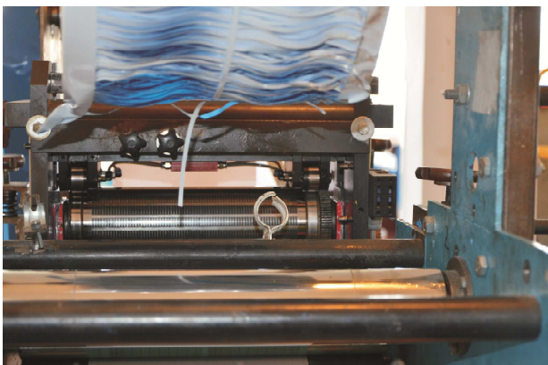
Fig. 12. The die cutting unit in a printing device.
