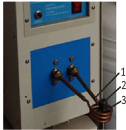
Fig. 2. Induction heat treatment of pinion type parts: 1 – helix inductor; 2 – pinion type part; 3 – hardening mixture AD applied to the active surface of the pinion type part.
