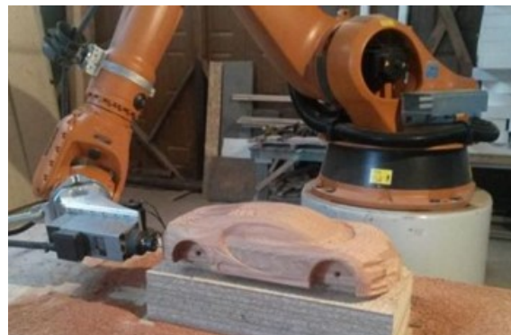
Fig.1. Industrial robot used in mechanical machining processes (milling, drilling, deburring).
