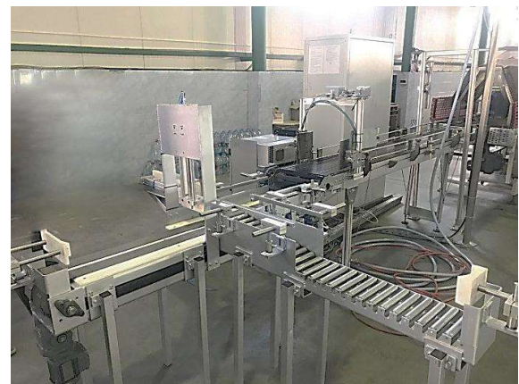
Fig. 14. The conveyor at the end of the bottling line.
