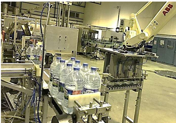
Fig. 16. The gripper mounted on the robot in phase of picking longitudinally arranged 2 packs of bottles.
