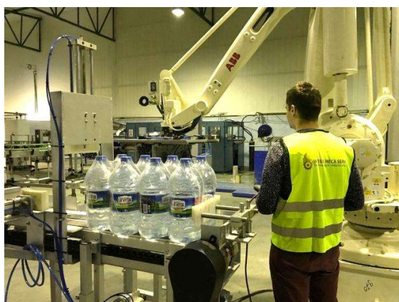
Fig. 17. Overall robotic cell programming and palletizing tests (the gripper mounted on the robot in phase of picking transversally arranged 4 bottles packs).
