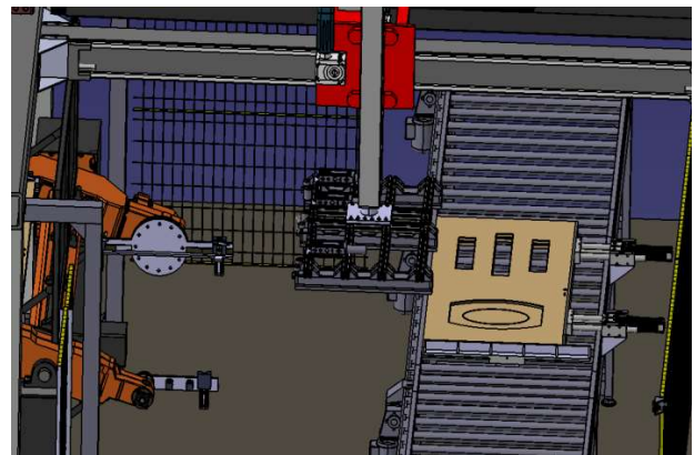
Fig. 12. Door transfer section.
