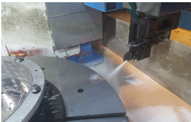
Fig. 9. Airplane turbine elements processing on a turning center.
