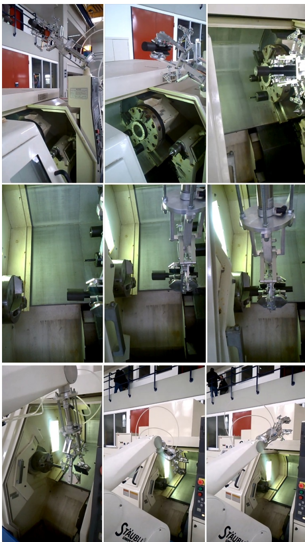
Fig. 11. Application example of CNC lathe loading.
