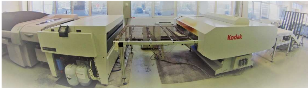
Fig. 2. Computer to plate line.
