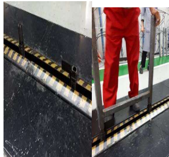
Fig. 11. Improvement – Bar conveyor.
