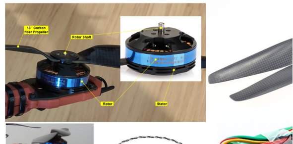
Fig. 3. Components of the hexacopter propulsion system currently mounted on drone frame.
