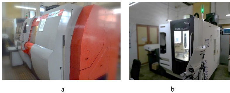
Fig. 2. ICPE's CNC machines from pilot experimental model: a – Emco Maxxturn 65; b – Dmg Mori CMX600V.
