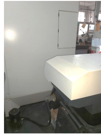
Fig. 7. Vibration monitoring of the emulsion pump (Dmg Mori CMX600V).
