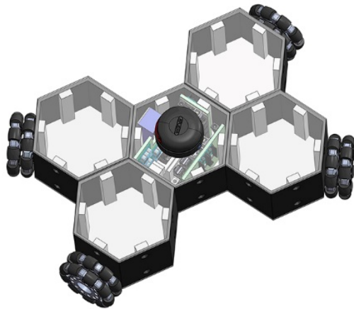
Fig. 9. Omnidirectional mobile robot with 4 Swedish wheels with rollers arranged at 90°.
