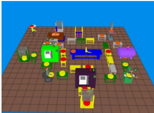
Fig. 14. Optimal location of P product resources made in Delmia Quest.
