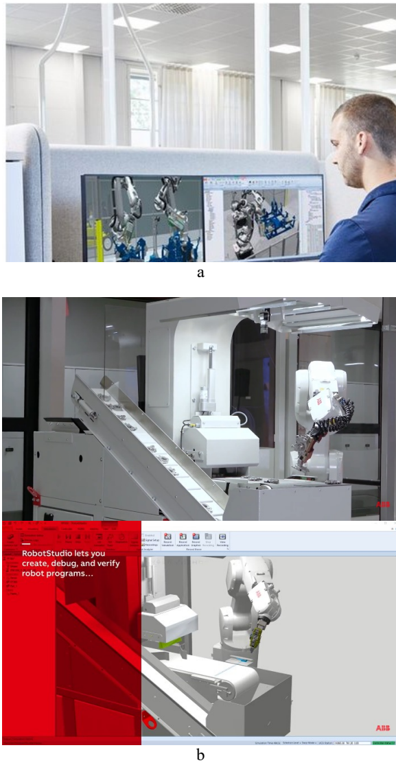
Fig. 5. Virtual commissioning work environment: a –Simulation interface [25]; b – Virtual commissioning comparison between ABB Robotstudio interface and reality [26].
