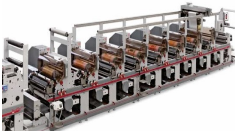
Fig. 2. Flexographic press used for printing with 8 printing units [9].
