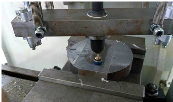
Fig. 4. Close-up of polishing jig mounted on cnc mill with rotating mandrel and ring shaped tool.
